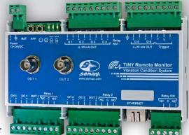
El TINY Remote Monitor (TRM) is two-channel equipment for condition controlling of machines by vibrations and temperature.
