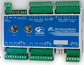
El TINY Remote Monitor (TRM) is two-channel equipment for condition controlling of machines by vibrations and temperature.
