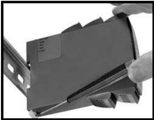
Image 1: Separate the DIN rail module by raising the upper lock.
