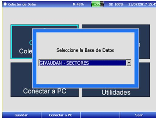
With ENTER key it opens the display list showing the different databases available, then it can be selected the correct one with navigation key, confirmed with ENTER key, and then activated F1 to save selection.
