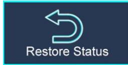
This utility is very important because it will allow the operator to return the status of a route already measured to a state not measured, in order to make a new measurement route without losing measurements already made.
