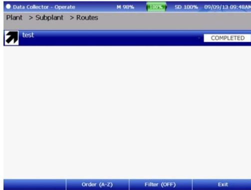
A measurement route is the grouping of multiple equipment on a sub plant, sorted according to collection.
