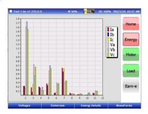
Harmonic components compare magnitude of harmonic components to fundamental currents and voltages of system. Bar chart displays distribution of content on different harmonic numbers for all currents and voltages.
