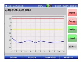
Above we see the title "Voltage Unbalance Trend", while on the bottom part we see graphically displayed the value of monitored quantity (y-axis) against test numbers (x-axis).
