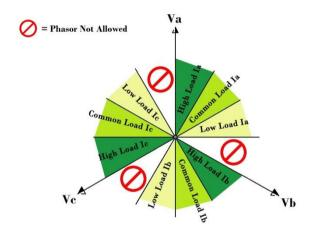
To get a correct setup, all three current phasors must be in the same area.
