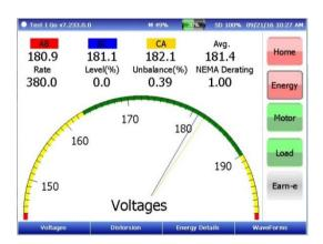
On the top with three different colors, we see voltages for voltage phasors. Also, on the top we see the Rate, Level (%), Unbalance (%) and NEMA Derating.
