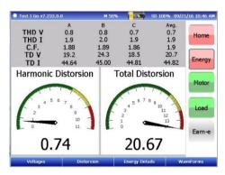
What this function does is examinate total harmonic distortion of three single phases to neutral voltages. The function compares level of total harmonic distortion to threshold values that you define.
