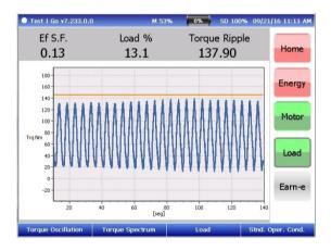
In addition, on top we see the Effective Service Factor, Load % and Torque Ripple.
