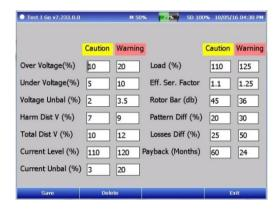
In this window we can define thresholds against which machines will be tested. In each test type, we must enter caution and warning thresholds. Using navigation keys, we can select any box we want to modify.
