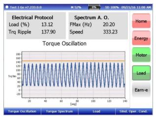
"Electrical Protocol" division on top left part of the window shows Load (%) and Torque Ripple. While Spectrum A.O., on the right side, shows the Fmax (Hz) and Speed.
