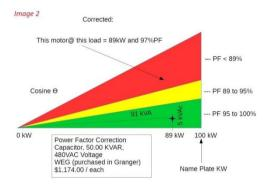
We can see that the amount of power provided by the motor is 89kW in both scenarios, but with the crucial distinction that when power factor is corrected the Apparent Power is 16kVA less, that is, motor consumes 16kVA less for the same amount of work.
